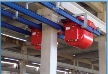
The Marcantonini concrete distribution system is the result of years of dedicated effort by our engineers to achieve maximum functionality, efficiency and reliability in the rapid transport of concrete. Marcantonini Flying Buckets can transport both wet and dry concrete in a fast (from 60 m/min to 240m/min) yet controlled way so that concrete arrives at its destination swiftly without changing any of its characteristics.
