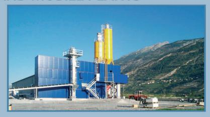
These compact, modular batching plants are easy to install and are ready for full production in a matter of hours. Each plant is either trailer mounted or containerised for transportation by road, rail or sea. Assembly is easy, complete installation and commissioning can be carried out in a maximum time of 2 days due to the unique design which negates the need for foundations or complex civil works.
